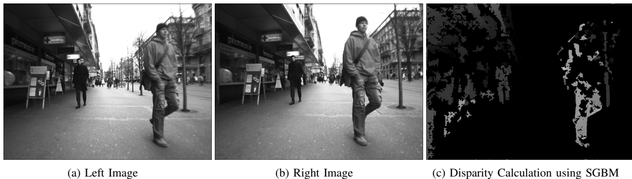
Fig. 2: Diparity Image Calculation form the two Stereo Images
